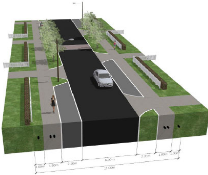
Diagram 5 - Local Road With Cyclepath
