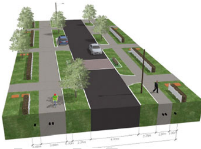
Diagram 5 - Local Road With Cyclepath
